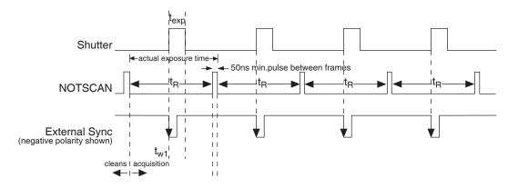
Figure 44. Overlapped Mode where  $t_{wl} + t_{exp} + t_c < t_R$
